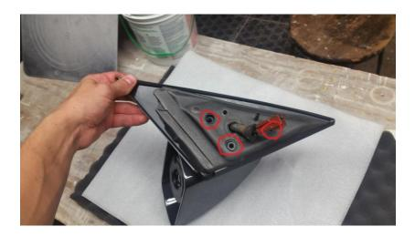
20. Install the new mirror glass into the new mirror housing by firmly pressing it into the mirror housing until it locks in place. Make sure that the cutout of the mirror glass backing is on the bottom of the mirror housing. See picture directly below. Note: the glass which contains the writing "Objects in mirror are closer that they appear" belongs on the passenger side mirror since it is convex glass and the driver's side mirror is not.
