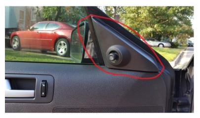
4. Once you have pulled the cover away from the car, disconnect the gray electrical harness by depressing the clip and pulling away. You can now put the cover in a safe place so that it does not get scratched or damaged while you perform the rest of the mirror install. The gray harness is circled in the picture discrets below:
