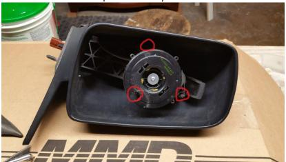
12. Use the flathead screwdriver or your finger to gently pull two (2) the clips away from the wiring harness that attaches the wiring harness to the mirror motor (there is one clip on each side). Be careful not to snap the clips from the harness – these do not require much force to remove. I have circled the plug and clips in the picture directly below (note: this picture displays the harness just after separation
