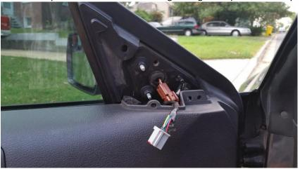
22. Using the 11mm socket and ratchet, reinstall the three (3) nuts onto the bolts. Plug in the brown wiring harness.
