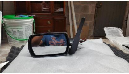
21. Line the three (3) bolts and the wiring harness on the new mirror housing up with the holes in the vehicle and push the new mirror housing through. See picture directly below.
