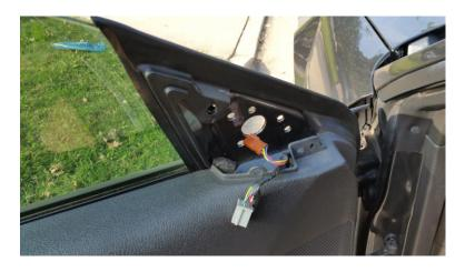
8. Place the old mirror onto a bench and remove the three (3) bolts with the 4mm socket and ratchet. The bolts do not require much force to remove. The bolts are circled in the picture directly below.
