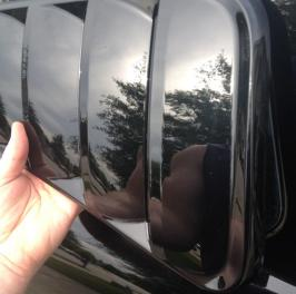
6. Peel stickers from back of window louver as they will be visible from the inside of the rear passenger seat if not removed before final placement.
