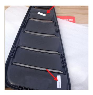
7. **Using only 1** of the supplied alcohol prep pads rub down the mounting points on the louver as well as the outside of the quarter window where the louvers will adhere to.
