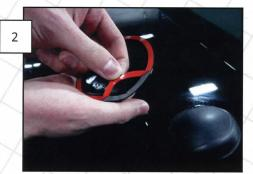
Remove the backing from the 3M tape on the back side of the cover as shown.
