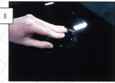
Be sure to center the cover over the factory antenna and place it on the decklid. Once the cover is properly located, firmly press down to full seat the adhesive tape.
