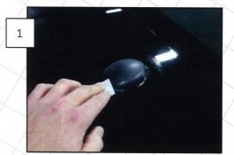
Clean the area around the factory antenna thoroughly with the supplied alcohol prep pad.
