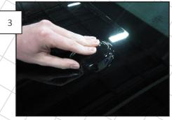
Be sure to center the cover over the factory antenna and place it on the decklid. Once the cover is properly located, firmly press down to full seat the adhesive tape.
