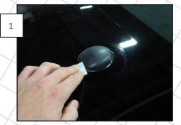
Clean the area around the factory antenna thoroughly with the supplied alcohol prep pad.
