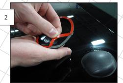
Remove the backing from the 3M tape on the back side of the cover as shown.
