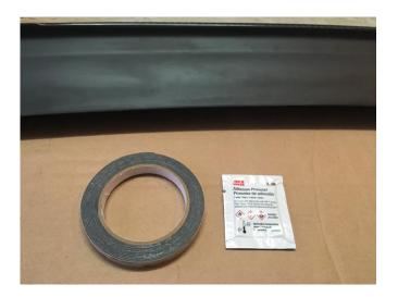
Attach 3M double-sided tape around the entire border of the bottom surface of the spoiler. NOTE: Prior to completion of the next step, it is recommended to try a dry fitting for alignment and sizing of the bolts. The provided bolts were too long for my installation, thus shorter bolts were required to be purchased and used instead. When all pieces appear to have proper fit, proceed with the next step for final installation.
