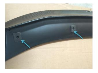
2. Wipe the border of the bottom surface of the spoiler with 3M adhesive promoter and allow to dry for 60 seconds.
