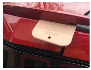
4. After successful removal of the spoiler, there will be adhesive tape still attached to the trunk. Carefully clean all remaining residue from the trunk using a scraper and adhesive remover. Applying LOW heat with a hair dryer or heat gun while scraping may assist in removal of the material. This step requires time and patience.
