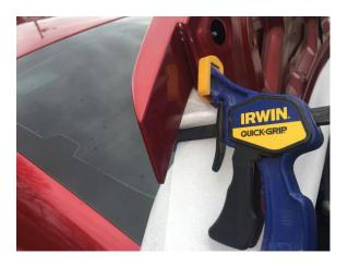
Using the 10mm socket wrench, loosen each of the 4 nuts securing the spoiler to the trunk lid. Two of the nuts are exposed by careful removal of black plastic plugs using a prying tool. After loosening, remove the nuts carefully while ensuring support of the spoiler to avoid damage to the vehicle.
