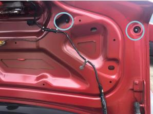
3. Close the trunk lid and carefully separate the adhesive material between the spoiler and trunk. This step requires patience and time to avoid scratching the paint of the vehicle. Combining Bondo scrapers and
