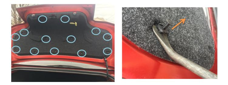
2. Remove the liner, being careful of the emergency trunk release lever and the trunk latch mechanism.
