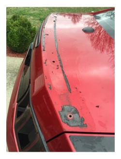
5. When all residue is cleaned from the trunk, wipe the area that the new spoiler will be applied using the alcohol pads.
