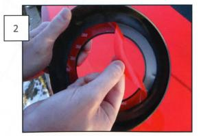
Remove the tape backing by pulling on the small tab as shown.
