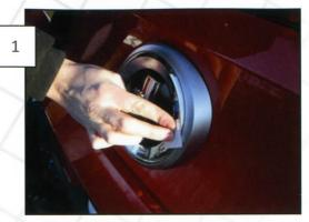
Using the supplied alcohol prep pad, thoroughly wipe down the chrome plated area of the emblem where the cover will adhere.
