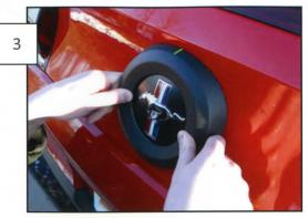
Install the cover over the emblem as shown, making sure the thicker wall (marked by a green line) of the cover is at the top. Once the cover is properly aligned, press down firmly around the edges to fully seat the tape.
