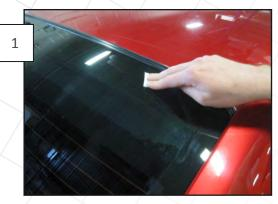
Wipe down the outer upper edge of the rear window with the supplied alcohol prep pads where the spoiler will adhere. Once dry, follow with the supplied 3M Adhesion Promoter.
