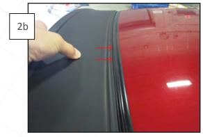
Pull the center of the spoiler up so it is even with the window weather stripping. Once the spoiler is properly located, press down firmly around the edges to fully seat the adhesive tape.
