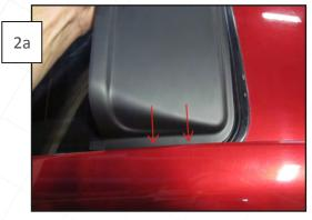
Peel the backing from the 3M tape and place the spoiler over the rear window (do not let the tape adhere yet). Tuck the outer edges of the spoiler into the quarter window trim as shown.
