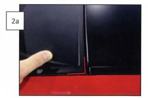
Peel the backing from the 3M tape and place the spoiler over the rear window (do not let the tape adhere yet). Line the upper corners of the spoiler with the upper corners of the rear glass as shown.
