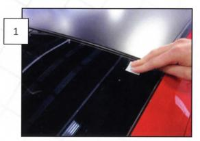
Wipe down the outer upper edge of the rear window with the supplied alcohol prep pads where the spoiler will adhere. Once dry, follow with the supplied 3M Adhesion Promoter.
