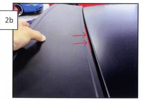
Then push the center of the spoiler up towards the back edge of the glass. Once the spoiler is properly located, press down firmly to fully seat the adhesive tape.
