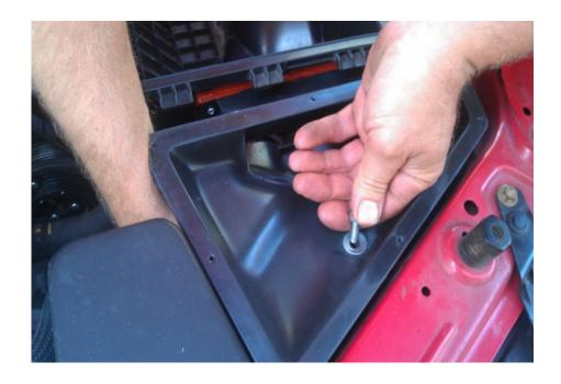
7. Place Billet Aluminum Grate on top of 90 degree adaptor elbow and install 7 Small Hex Head screws with 5/64" or 2mm Allen Wrench.
