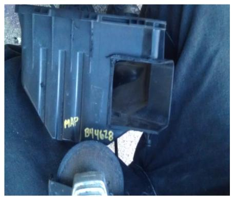
2. Using a grinder level out the first 3 support ribs and any bumps left over from cutting in the step before as shown below.
