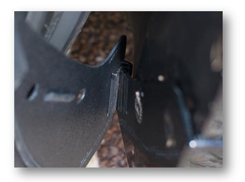
**Step 5:** Make sure the holes align with the holes in the rocker panel. Insert the pin/clip into each hole and press it in until it is completely flush.
