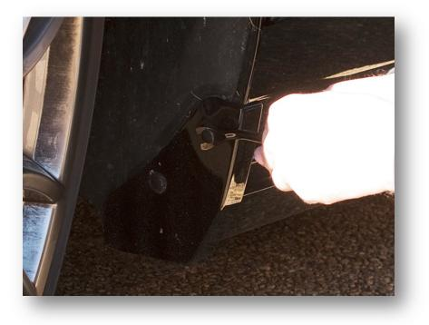
**Step 4:** Align the back grove on the Splash Guard with the back of the rocker panel and then align the top with the fender overlap.
