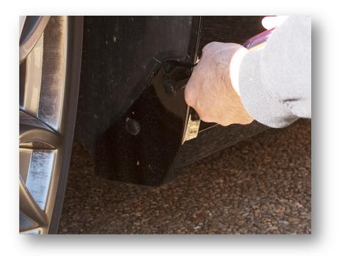
**Step 3:** Using the clip remover tool pry both of the pin and retainer clips out.
