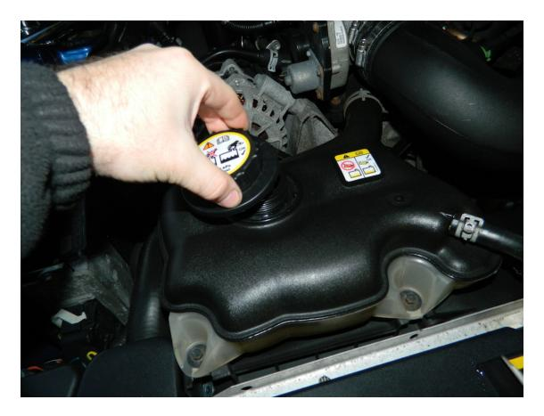
Prior to adding additive it's good idea to test coolant mixture for correct ratio and protection. Using an antifreeze tester check coolant for a 50% coolant to 50% distilled water solution mixture. The 50/50 mixture is recommended for year round giving a -35°F to 223°F protection.
