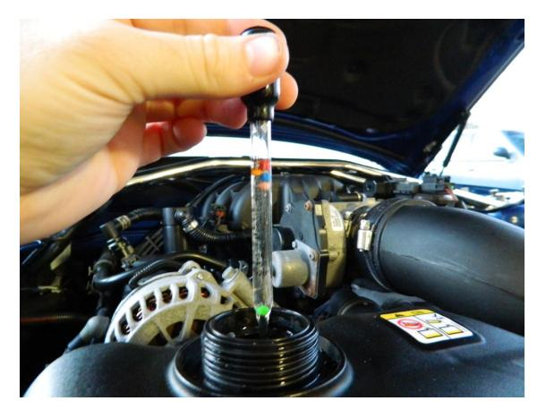
3. Inspect reservoir fluid level, if filled to "Cold line range" or above removal of coolant is required. Using a suction gun remove at least 16 oz. of coolant from reservoir.
