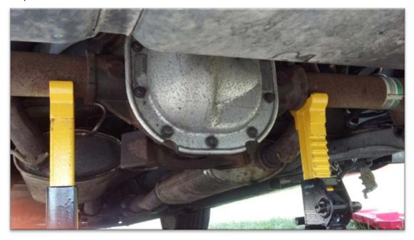
3. After you get the car in the air remove both rear tires to gain access to the bolts that hold the rear sway bar onto the lower control arm. The bolts were in the two holes shown below and are ½ inch in size. \*Note: it would be easier to do this with someone holding the sway bar while you loosen it up.
