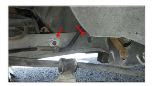
4. Now you need to pick a side to work on and locate the 13/16 inch bolt and nut that attach the lower control arm to the axle housing. This is probably going to require the use of PB blaster and your breaker bar. These are the tightest bolts you are working with during the install.
