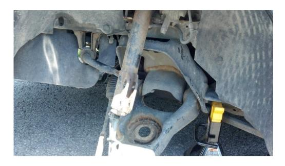
10. Transfer or replace the spring isolators onto the new spring.
