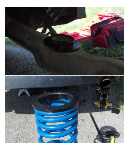
8. Position the new spring and slowly jack the lower control arm back up into place. Replace the bolt to secure it back to the axel housing. Bolts should be put on at 111ft/lbs and held with red loctite.
