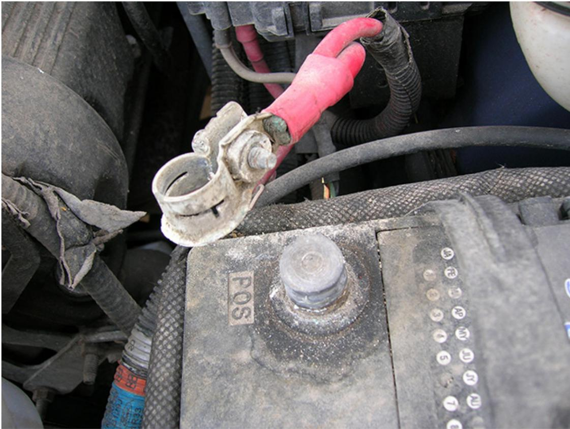
11.) When you are finished filling the coolant reattach the positive battery connection and you are ready to take the car out for a drive. Make sure that you have added enough coolant as air pockets will work their way out after a good drive.
