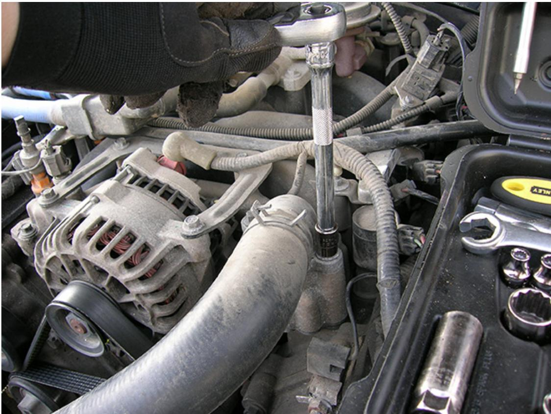
4.) Pull off the thermostat housing and hose. You can disconnect the hose from the housing. To this you will require vice grips or pliers to pinch the metal clamp and slide the hose off. This is not necessary.
