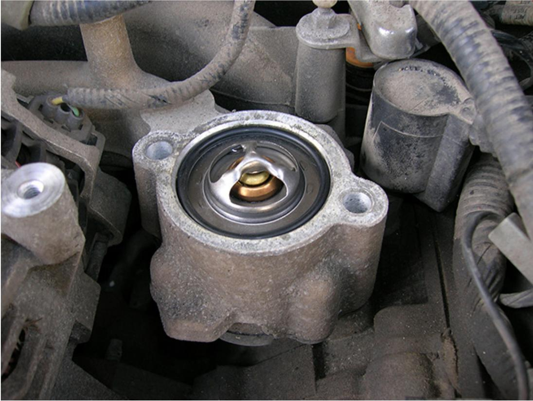
7.) Now get your torque wrench. Set it to 18 ft/lbs or 25 Nm. Put the housing back on and tighten up the bolts.
