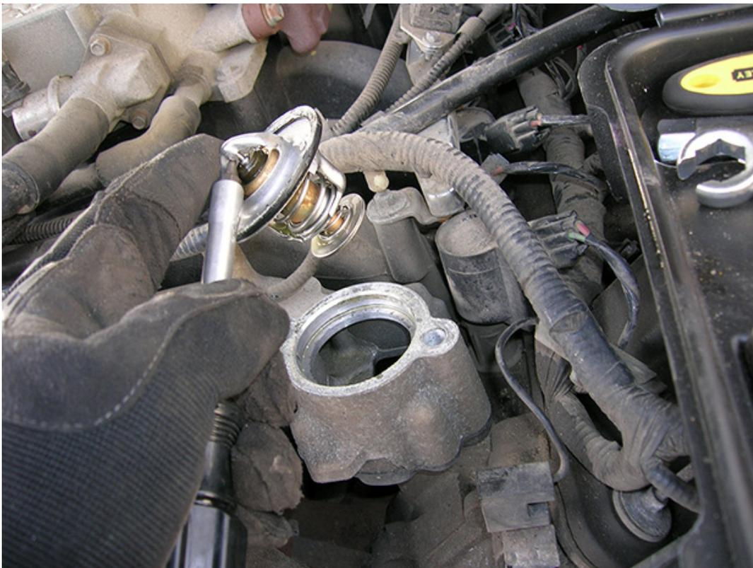
6.) Place new thermostat and o-ring into where the old thermostat was. If you push down on the thermostat, it will pop into place. It will not stay exactly where it was because the spring will push it back up. Make sure the o-ring is in position for a good seal.
