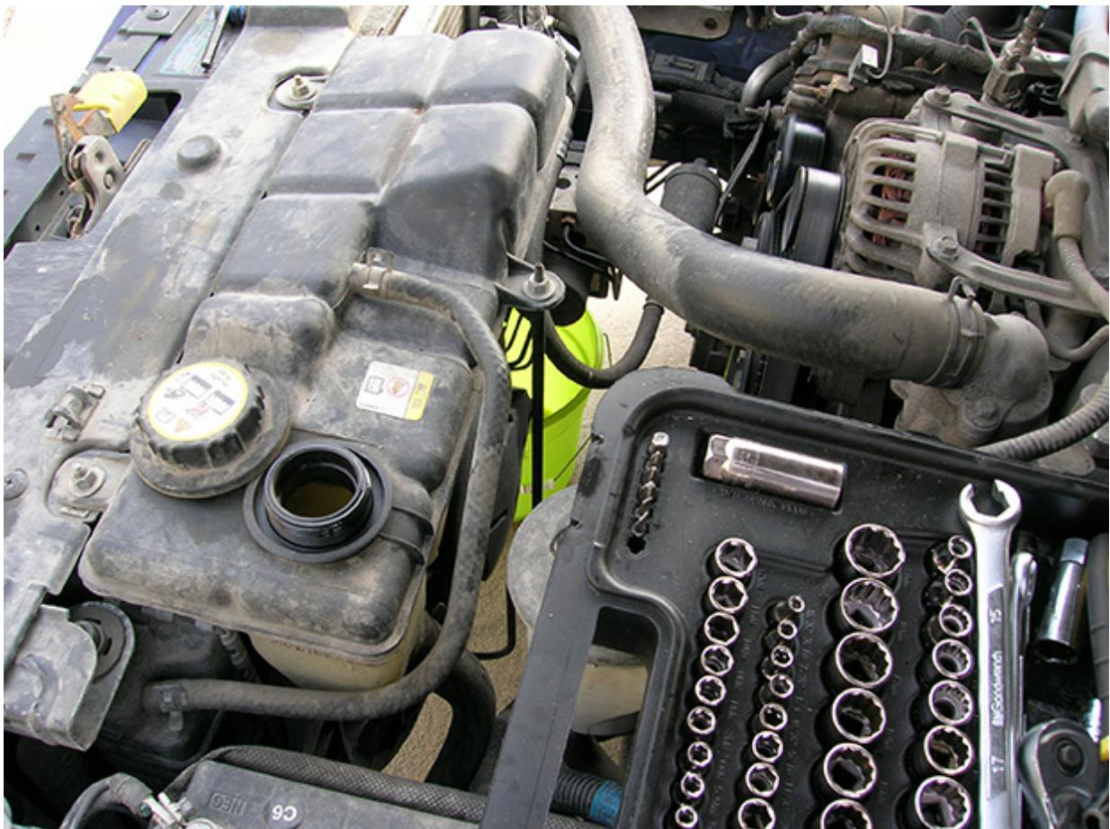
2.) Get your 10 mm socket, an extension and your ratchet. Undo the alternator bracket bolts. Remove the bracket.
