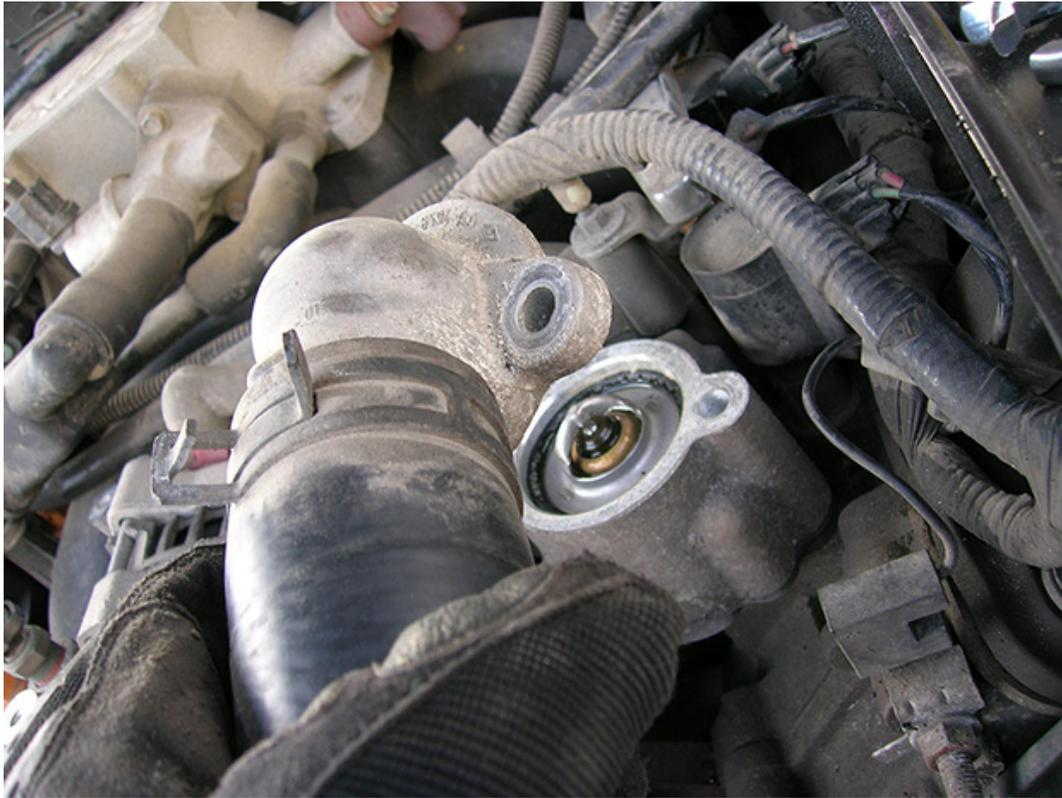
5.) Use a screwdriver to carefully pull the old thermostat out. Be careful not to indent the housing. Vice grips may also work well for this step.
