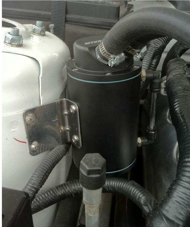
6. Locate the PCV fitting on your cold air intake. Connect the hose to the fitting with the supplied hose clamp and a flat head screwdriver.
