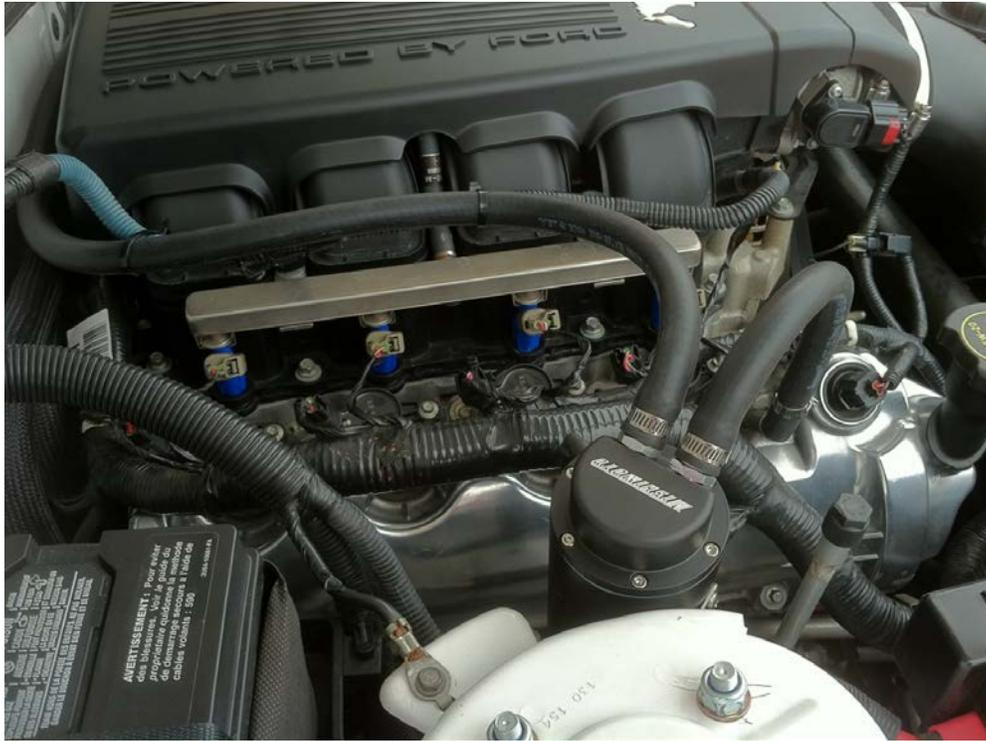
8. Run some more hose from the oil catch can to the PCV valve. Cut to length and attach with the supplied hose clamps, using a flat head screwdriver to tighten. I ran mine to the passenger side PCV valve.
