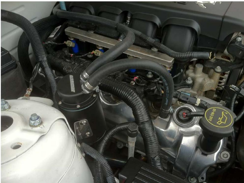
9. For upkeep: use the hose on the side of the catch can as a fluid level reference to let you know when to drain. If the line is over halfway full, it is time to drain it out. To empty the contents, unscrew the drain plug from the bottom and reinstall once drained.
