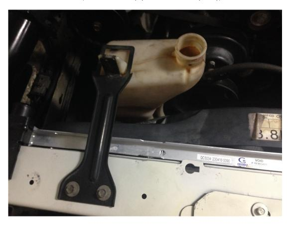
6. Next is the cooling fan which is held in by two 8mm bolts, one on each side and an electrical connection in the middle. (Fan will then lift right out)
