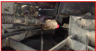
7. Lastly, there are two brackets with a single 8mm bolt holding the radiator in place.
