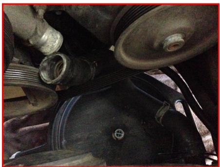
5. The reservoir is held in by a bracket with two 10mm bolts. Once the bolts are out twist the reservoir to one side and lift it out. (remember to empty the reservoir completely)
