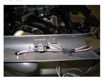
The pillar's "bullets" are designed to house 2 1/16" gauges. Autometer is the brand of choice at Speed of Sound, and exhibit a perfect fit. Should your gauge require a more snug fit, simply attach a samll piece of Velcro (only one side, hook or loop, about the size of half a postage stamp) or a single wrap of electric tape at the rear of the gauge. This will ensure a firm fit.
