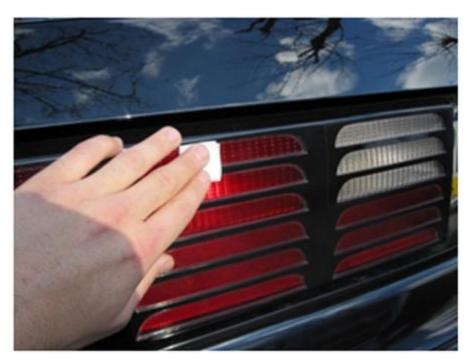
2. Peel away the backing from the Velcro strips. Align cover carefully over tail light, but do not fully press down yet. Once the cover is centered over the light, firmly press down to fully seat the adhesive backing. Repeat for opposite side to complete the installation.
