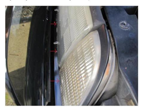
2. Once the cover is secured between the light housing and bumper cover, push the top part towards the headlight and tuck it under the radiator support as shown. Repeat for opposite side to complete the installation.
