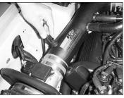
30. Reconnect the mass air sensor and air temperature sensor electrical connections.
