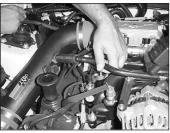
28. Install the PCV line into the 3/4" ID vent hose.
