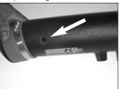
19. On models equipped with an external air temp sensor install the grommet into the hole in the previous step.
