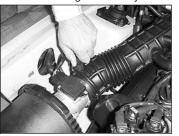
2. On models equipped with an external air temp sensor, disconnect the air temp sensor electrical connection.
