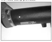
18. On models equipped with an external air temp sensor, drill out the drill point using a 11/16" drill bit.
