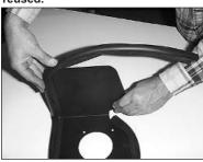
13. Install the trim seal onto the heat shield. NOTE: some cutting and trimming will be necessary to achieve best fit.
