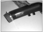
17. Attach the silicone straight hose (08630) to the K&N intake tube using the hose clamp provided.
