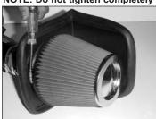
22. Attach the air filter element to the adapter using the hose clamp provided.
