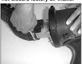
9. Loosen the hose clamp and detach the intake tube from the mass air sensor.
