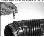
10. On models equipped with an external air temp sensor remove the air temperature sensor from the intake tube.
