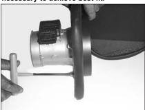
14. Assemble the mass air sensor, heat shield and adapter, using the gaskets and hardware provided as shown.
