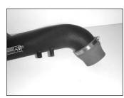
16. Attach the silicone step hose to the K&N intake tube using the hose clamp provided.
