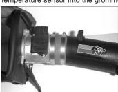
21. Attach the K&N intake tube to the flange on the mass air sensor using the hose clamp provided. **NOTE: Do not tighten completely at this time.**
