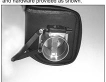
15. Attach the brackets to the mass air sensor as shown.
