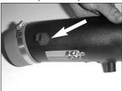
20. On models equipped with an external air temp sensor, insert the air temperature sensor into the grommet.
