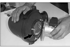
12. Remove the mass air sensor from the air cleaner.
