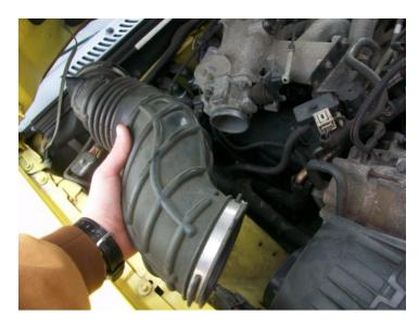
5. Using an 8mm wrench, loosen and remove the bolt holding the air box to the engine bay.
