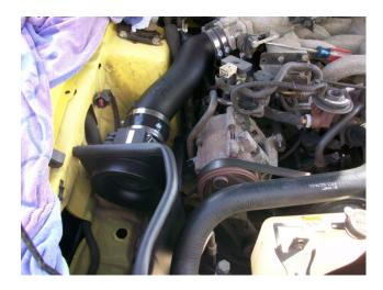
20. Line up the previously attached bracket and the holes on the A/C compressor. Reattach and tighten the bolts that were taken out in step Eleven.
