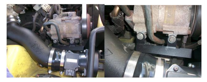
21. Attach the filter element to the adapter ring using the supplied large hose clamp.
