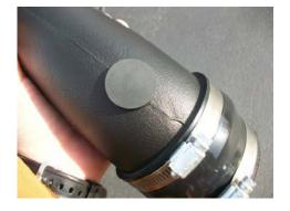
16. Screw in supplied plastic vent hose port into intake tube using a 9/16" wrench.
