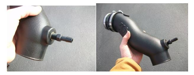
17: Attach intake tube to mass Air flow sensor using a flat head screwdriver to tighten the hose clamps.
