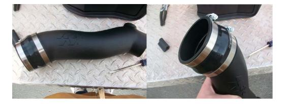
15. On 2001-2004 models, Plug the hole in the Intake tube with supplied plug.
