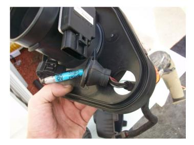
10. Using a 10mm Wrench, Remove the two bolts holding the mass air flow sensor on the old intake case. Remove the Mass air flow sensor this is going to be re-used in the new Intake.
