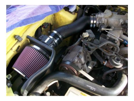
22. Reconnect the wiring harness to the Mass airflow sensor and tuck the excess wiring inside of fender.
