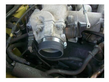
19. Lower in the assembled intake and connect the intake hose to the throttle body.
