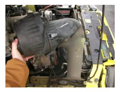
7. Unclip the two clips holding the air box together and separate the two pieces.
