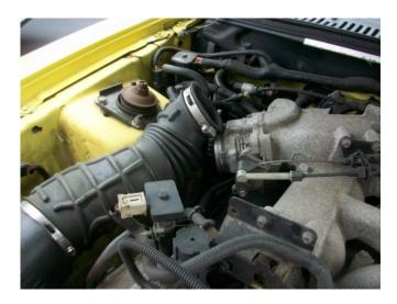
4. Using a flathead screwdriver, loosen the hose clamp connecting the intake hose the filter box.
