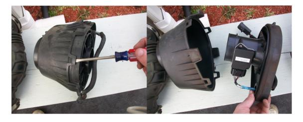
9. Push the Wiring harness through the hole and set it aside for later use. (TIP: Try to pinch and twist the seal to get the harness through.)
