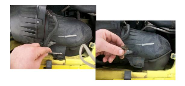
6. Pull the Air Box out of the fender well and up out of the engine bay.
