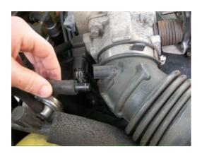
3. Using a Flat Head Screwdriver, Loosen the hose clamp connecting the air intake hose to the throttle body. Disconnect the tube from the throttle body.
