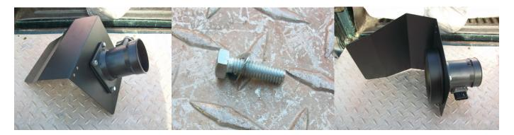
13. Attach the Supplied Bracket to the heat shield with remaining 6mm hex bolts and flat washers.
