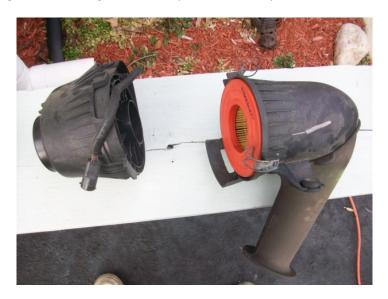
8. Using a flathead screwdriver, pry the tabs holding the case together open. Separate the two pieces exposing the mass air flow sensor.
