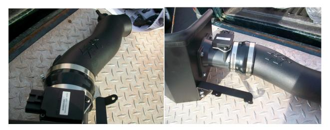
18. Attach silicon hose to throttle body with supplied hose clamps. Tighten using a Flathead screwdriver.
