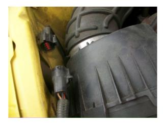
2. Disconnect the hose on the existing air intake tube.
