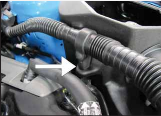
p. Plug the rubber support into the hole of the AEM® airbox as shown.
