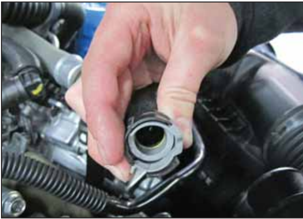
g. Release the crankcase vent tube from the nipple. Slide the gray clip to the side and pull on the connector to release it.
