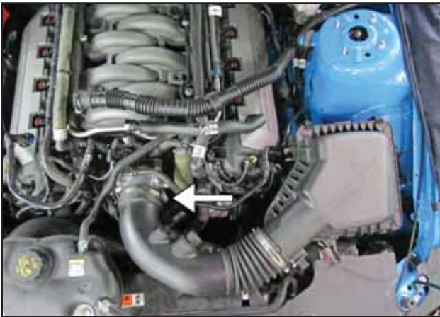
i. Loosen the hose clamp on the throttle body.
