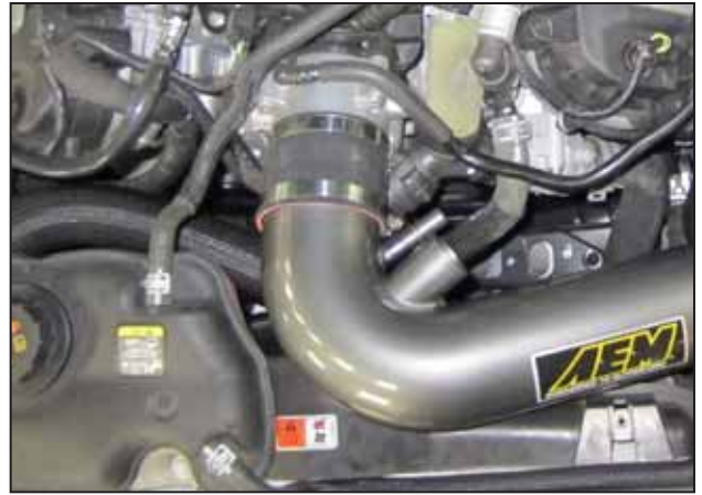
m. Insert the end of the AEM® intake pipe into the throttle body coupler as shown.
