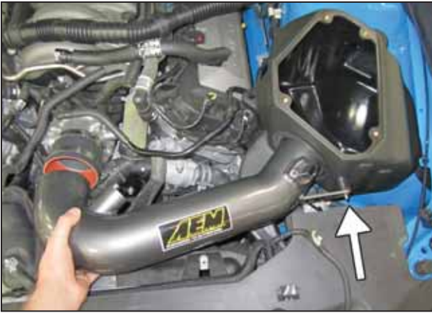
l. Install the AEM® intake pipe as shown. Make sure that the bracket engages the stud on the rubber mount.
