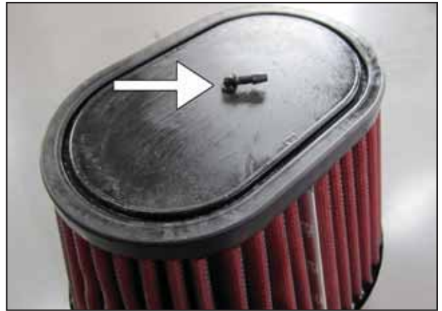
q. Insert the 90 degree plastic connector into the hole located on the air filter top.
