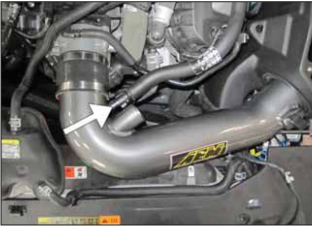
n. Connect the OEM crankcase vent line to the AEM® intake pipe by firmly pressing the connector onto the nipple until it 'clicks' into place.
