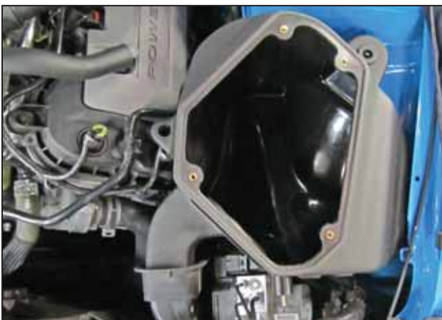
j. Guide the two bosses on the bottom of the AEM® air box into the grommets installed in step 3g.
