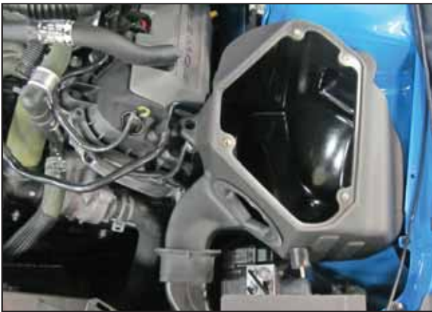
h. Lower the AEM® airbox into position as shown.
