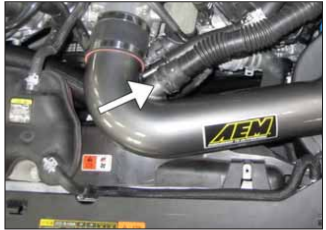
o. Connect the sound tube to the AEM® intake pipe and secure it in place with the OEM spring clamp.
