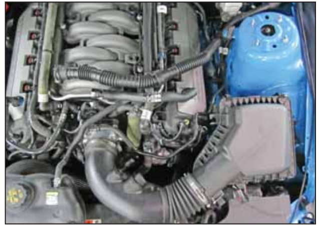
h. Position the sound tube and crankcase vent tube out of the way as shown.
