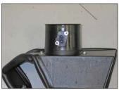
13. Install the mass air sensor into the K&N $^{\odot}$  mass air sensor housing and secure with provided hardware.
