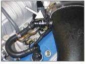
22. Connect the crankcase vent line to the quick disconnect fitting installed into the K&N $^{\!0}$  intake tube.
