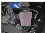
24. Install the K&N  $^{\! \odot}$  air filter and secure with the provided hose clamp.
