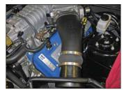
21. Install the K&N® intake tube into the silicone hose at the throttle body and align with the mass air sensor housing. Slide the silicone hose down the K&N® intake tube onto the mass air sensor housing. Align the tube for best fit and then secure with the provided hose clamps.
