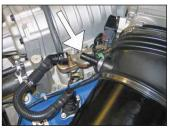
5. Rotate the locking ring and then disconnect the crankcase vent hose as shown.
