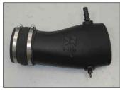
20. Install the provided silicone hose (08695) onto the  $K\&N^{\otimes}$  intake tube, slide the hose all the way onto the  $K\&N^{\otimes}$  intake tube; do not tighten at this time
