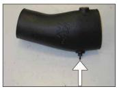
17. Install the provided 3/16" vacuum fitting into the  $K\&N^{\circledcirc}$  intake tube as shown.
