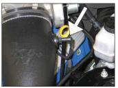
23. Connect the vent line to the 3/16" fitting installed into the  $K\&N^{\odot}$  intake tube.
