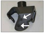
15. Install the factory mounting grommets to the two mounting posts installed on the  $K\&N^{\oplus}$  heat shield assembly as shown.
