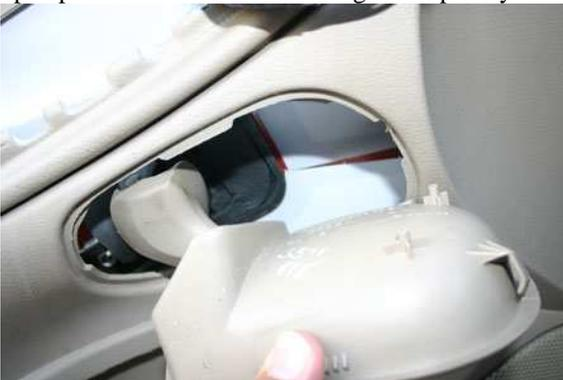
7. Remove the roll pin from the top of the handle, and discard original pin. The door handle can now be removed from the handle receiving assembly. Be aware of the return spring which will be re-used with the new handle, as well as the orientation of the spring.
