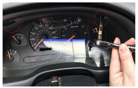
3) Carefuly remove your dash board cover by pulling it out. The dash board cover have 5 plastic stud so you need to take your time to corecly remove it.
