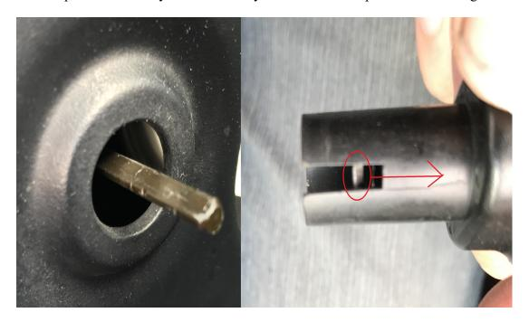
2) Remove the 7mm bolt from the dash board with your 7mm socket
