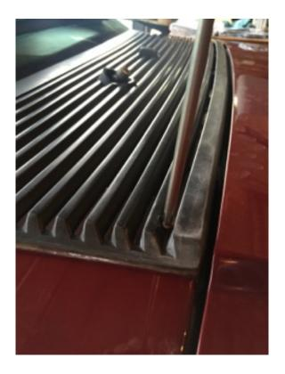
Step 6: After removing the 6 screws lift the cowl up, you will see a hose going to the sprayer.
