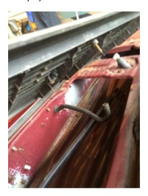
Step 8: With the cowl now free from the car, take a Philips screwdriver and remove the one screw holding the sprayer onto the cowl.
