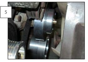
Separate the fan from the water pump pulley by pulling it toward the radiator. Remove all 3 stock pulleys, by pulling them toward the front of the car and replace them with the 3 aftermarket pulleys.
