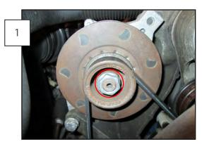
With the belt still attached, loosen the 15/16" nut in the center of the alternator pulley. Leave the nut loose, but in place.
