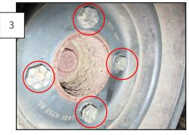
Loosen the (4) 9/16" crank pulley bolts in the crank pulley.
