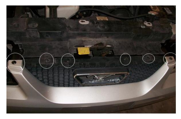
E. Now, release the bumper tabs from the header nose panel and pull the bumper off and set aside. To release the tabs from the headlight nose panel, you can use the Philips screw driver to pry open the slit in the headlight nose panel enough for the tabs to be released.
