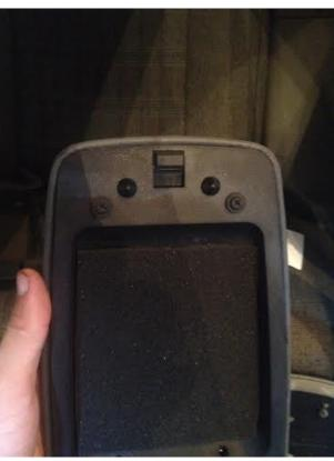
**Step 3:** Take the pad and trim and align it with the console bracket, The bracket should slide between the Arm rest pad and the trim.
