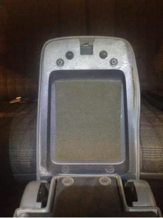
**Step 2:** Next taking the Phillips screwdriver unscrew the screws holding the armrest pad onto the trim and Armrest bracket, There should be 4 total.
