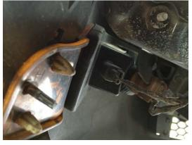
21. Re-install the 10mm bolts connecting the bumper to the frame
