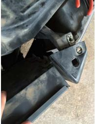
12. Remove 3 phillip head pin screws located on the inner splash shield. **NOTE**: From now until specified, removal shall be done identical to both sides of the vehicle.
