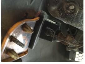
14. Using a 10mm socket, remove to bolts that connect the bumper the frame. They are located directly above the turn signal light
