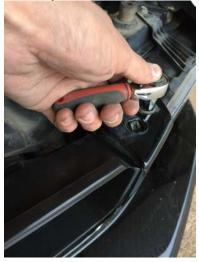
23. Re-install the 6 push pins on the radiator cover
