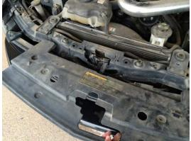
10. Using a 10mm socket, remove the two bolts connecting the bumper to the vehicle
