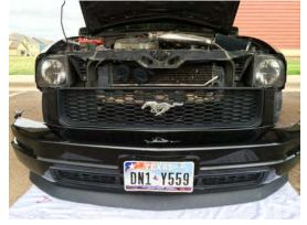
16. Using a flat head screwdriver, pry out the tabs keeping the stock grill in place. Be careful not to damage the connecting opening for the new grille
