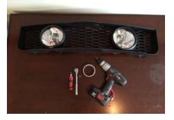
2. OPTIONAL: Unscrew four screws holding in the fog lights
