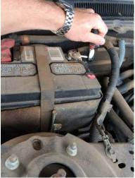
8. Using a flat head screwdriver, pop out the 6 push pins that keep the radiator cover attached
