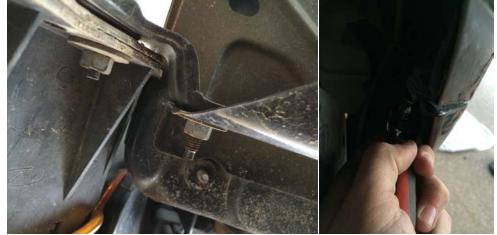
22. Push the bumper over the stopping pin and re-install the 10mm bolts connecting the grill portion of the bumper to the body
