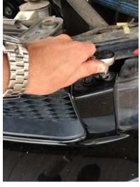
11. Once the bolts are removed, lift the bumper up and over a small stopping pin
