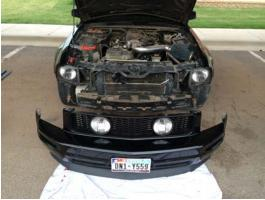
19. **NOTE**: Due to clearance issues you must snip a tiny piece of the fog light housing off and slightly bend the horn bracket for correct fitment. Once done the grill should snug.
