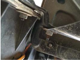
15. Now, all bolts are successfully removed, you can remover the entire front bumper. Be sure to place a towel or blanket on the ground so the bumper is not scratched
