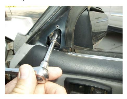
5. Remove the nuts from the mirror studs and then pop the mirror connection free from its mounting location.
