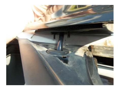
7. Connect the new mirror to the factory harness and secure it to the door in factory location.
