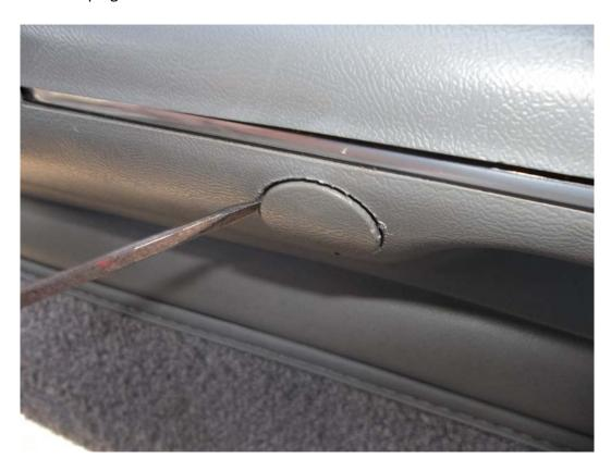
2. Remove the two 10mm bolts that secure the arm rest to the door. After this is done you will want to remove the three Philips head screws that are on the door panel one is located on the rear of the arm rest one on the speaker grill and the one that secures the door handle bezel.
