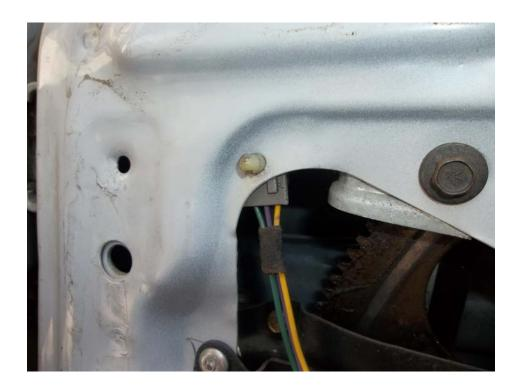
6. Unplug the mirror connection then simply just pull the mirror free from the door. Once removed take the new American Muscle mirror and fish the new mirror connector through the hole in the door then slide the new mirrors studs into the mounting holes. Once it is in place start the two 9mm nuts on the studs don't tighten this is to prevent mirror from falling out.
