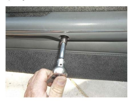
3. Remove the door handle bezel then remove the single Philips head screw that secures the access panel to the back side of the mirror.
