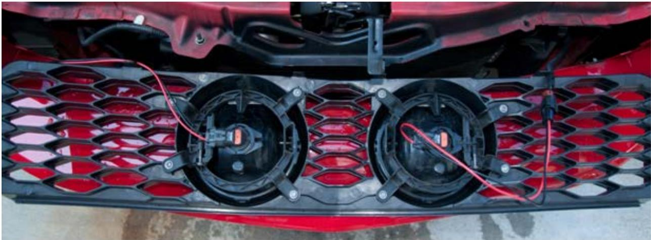
7. This is a good time to reconnect the negative wire to the battery and test your lights to ensure all connections are secure and functional.
