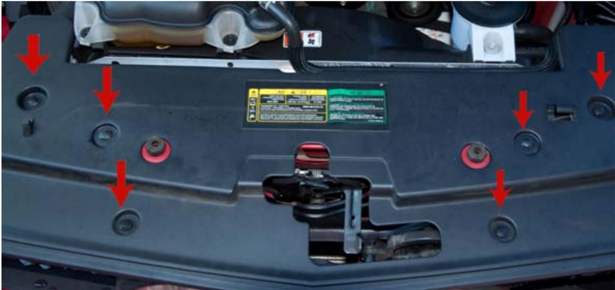
3. After removing the radiator cover, locate the (8) plastic tabs that hold in the stock grill and remove. You may need to gently bend the “female” part of the tab over the “male” portion to free the grill. Please see photo below for the respected locations of the tabs.
