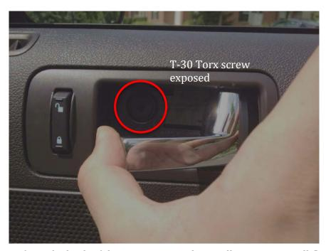
2. Remove the cover from the back of the armrest-area door pull. Use your small flathead screwdriver or trim panel removal tool to pry it forward approximately ¼ inch away from the door panel, then lift it straight up, to release it. Remove the T-30 Torx screw behind it.
