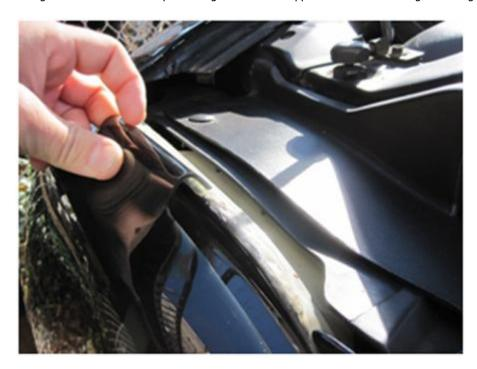
3. Once the tab is over the housing, push the cover back towards the light to fully seat the tab as shown:
