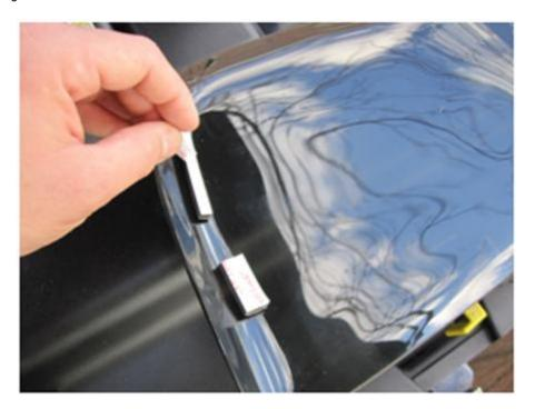
3. Place the cover over the light housing carefully to align it, but do not press down yet. Once the cover is centered and properly aligned, press down firmly to fully seat the adhesive. Repeat for opposite side to complete the installation.
