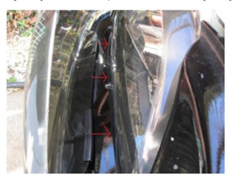
2. Push the top of the light cover towards the top of the light and lift the upper tab over the headlight housing as shown:
