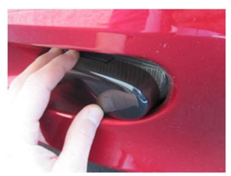
2. Push the top edge of the light cover over the top of the fog light as shown. Repeat for opposite side to complete the installation.
