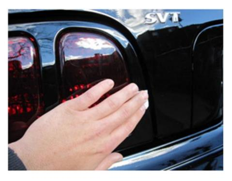
2. Peel the backing from the Velcro tabs as shown:
