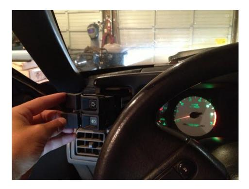
3. Reinsert the switch back into the bezel by pushing until you hear a click, this will let you know that it is inserted correctly.
