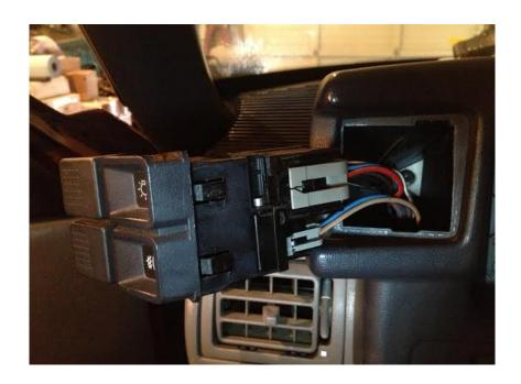
2. After removed disconnect the two connectors on the back of the switch.
