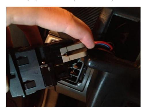
2. After plugging the two connectors back in turn on your key and test the headlight switch to make sure everything is in working condition.
