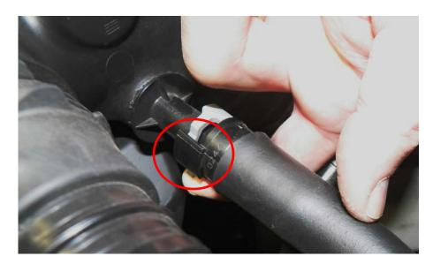
**Part 3: \*\*Automatic Transmissions Only\*\*** If you have an automatic transmission, there will be another smaller fitting next to the valve cover vent tube. To remove it, push down on the yellow tab while pulling away from the pipe fitting.
