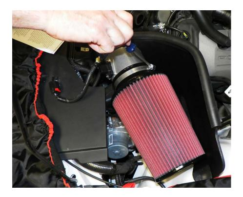
**Part 3:** Re-insert the factory round noise-transmission tube into the new inlet pipe assembly. Slide the hose entirely over the connector. Use a channel lock wrench to secure the factory spring clamp.
