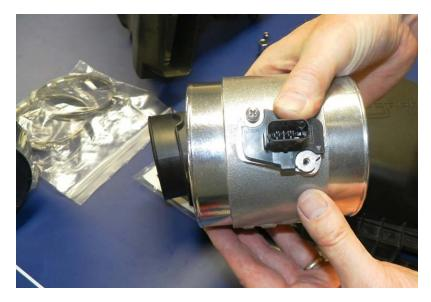
**Part 3:** If not pre-attached in the kit, attach the C&L airflow housing to the round end of the inlet tube using the supplied 4" hose clamps. For proper orientation, the sensor should be pointing towards you (or front of vehicle) and the C L stamp on the housing will be facing down. **NOTE:** Be sure to press the silver housing flush to the black MAF body.
