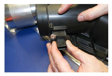
**Part 2:** Examine the silver aluminum C&L housing provided in the kit. If there are screws in the housing, remove them and set aside. Carefully insert the sensor cartridge into the aluminum C&L housing. When properly oriented, the sensor screw holes will line up correctly. Using the screws provided in the kit (not the factory screws), tighten the sensor cartridge.
