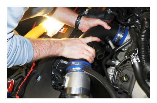
**Part 2:** Slide the C&L filter over the aluminum housing of the new MAF body. Orient the hose clamp for easy access to tighten. **NOTE**: At this point adjustments can be made; however, if the filter is bumping against the ABS lines, additional clearance can be made by bending the line slightly toward the front of the vehicle. This was not necessary on this installation.
