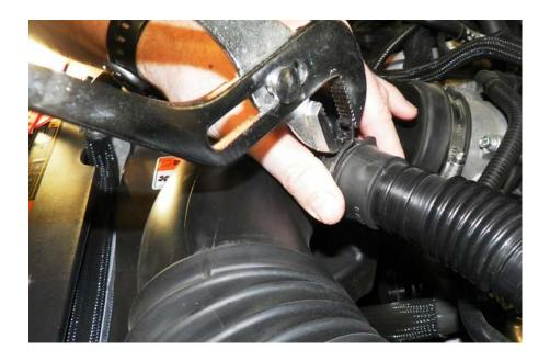
**Part 5:** Disconnect the flexible noise tubing from the factory air box by opening the rubber clamp that wraps around the tube. Move the noise transmission tube by pulling it away from the triangular shaped mount on the driver side strut tower.
