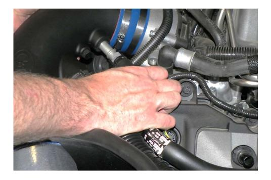
\*\*For Automatic Transmissions Only\*\* Re-use the original rubber hose that attached to the factory inlet tube. Pull back the plastic conduit and cut the hose just after the factory nylon release fitting. The exposed 3/8" rubber tubing will then slide over the barbed nipple previously installed.
