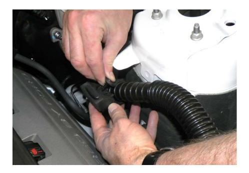
**Part 7:** Once all the fitment and adjustments are made, tighten all hose clamps firmly. Re-install the factory engine cover. Re-attach the strut tower brace if equipped.
