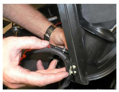
**Part 4:** Lift the stock air box slightly upwards and toward the rear of the vehicle. This will release the rubber feet that hold it to the vehicle. Slide the lower half from the fresh air feed that enters from between the headlight and radiator support. Remove the entire stock air box from the engine compartment.
