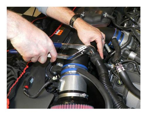
**Part 4:** Reconnect the valve cover vent tube on the new inlet tube. It will be secured by the locking tabs and click in place. **NOTE:** If there is difficulty or resistance connecting the vent tube, disconnect the tube from the valve cover and connect the inlet tube first, then re-connect the tube to the valve cover.
