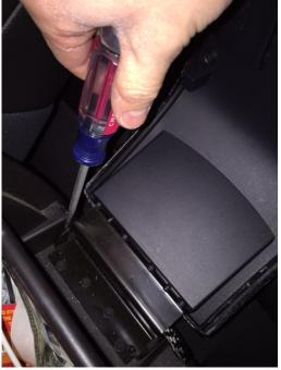
6. The back of the Trucarbon cover has prongs similar to the stock cover. The prongs on the Trufiber piece are metal and can bend to ensure a custom fit.Without taking the backing off the adhesive, make a couple of trial fits while gently bending the prongs to fit your vehicle. Once you find a nice fit, remove the adhesive backing and install.
