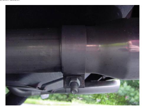
7. The next set of instructions is a bit confusing as well as slightly frustrating. Taking your time will save you a lot of time and effort. Slide the over-axle pipe over the axle and then fit it onto the end of the resonator. (Do not forget to place a band clamp over the pipe as well.) The over-axle pipe is pictured below with the resonators in the background.
