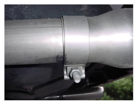
15. If a pipe does not stop leaking, fix as much has you can and then just drive the car around for about ten minutes. Usually, the pipes will heat up, expand, and stop leaking. The connections in the pipes will sometimes seal themselves. Remember, that just because it is not shooting water out, does not mean that it is still not leaking exhaust gases. Use some soapy water in a squirt bottle and spray it on the pipe and then look for air bubbles to indicate a leak.
