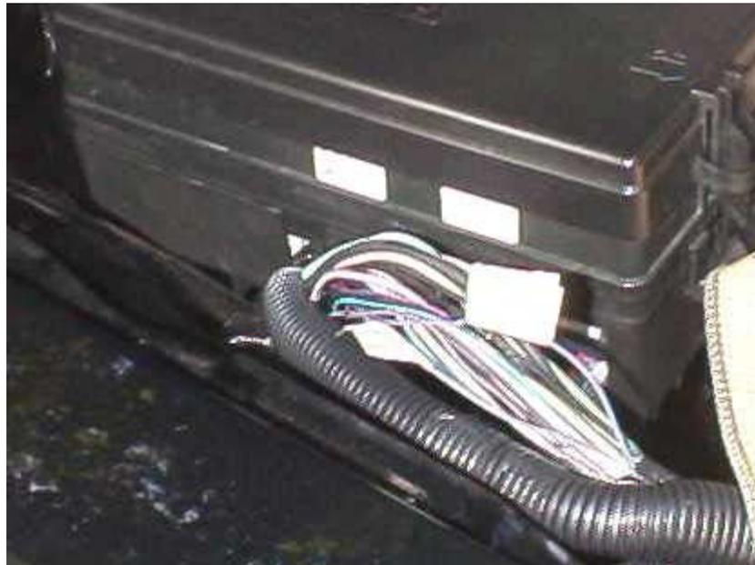
2) Open wire loom "A" (if necessary, remove or carefully cut any electrical tape to increase access to the wires).
