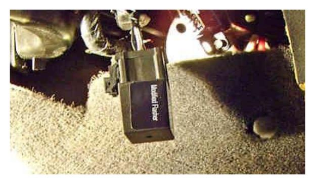
4. Reattach the modified flasher unit to the bracket underneath the dash.
