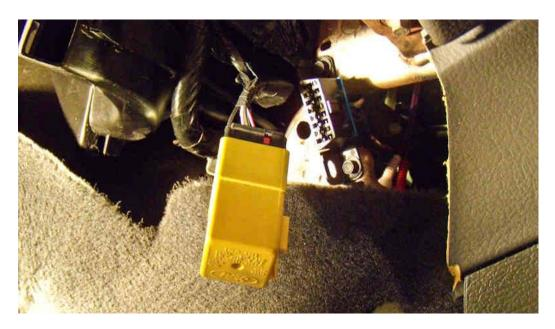
3. Unclip the yellow OEM flasher unit and replace it with the Raxiom Modified Turn Signal Flasher. Be sure to line up the blade connectors in the same manner as the OEM unit.
