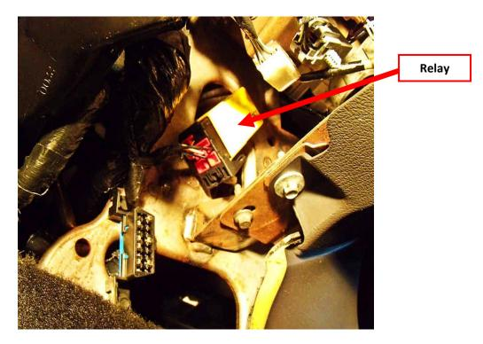
2. Pull the yellow relay unit down towards the OBD II port and out of the bracket holding it in place.
