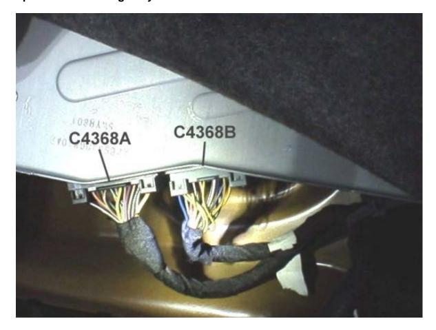
2) Unplug connector C4368B and unwrap it to expose the wires. Make the following connections:
