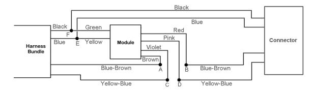
Using the diagram above, make the connections as follows:
