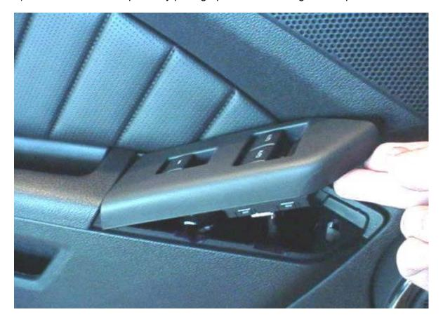
3) Unplug the connector on the rear window switch. Unwrap the tape to expose the harness wires.
