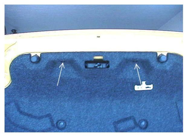
2) Reach up to the third brake light and disconnect the 2-pin connector. You must press the retaining tab to release the lock as you pull the connector straight back.
