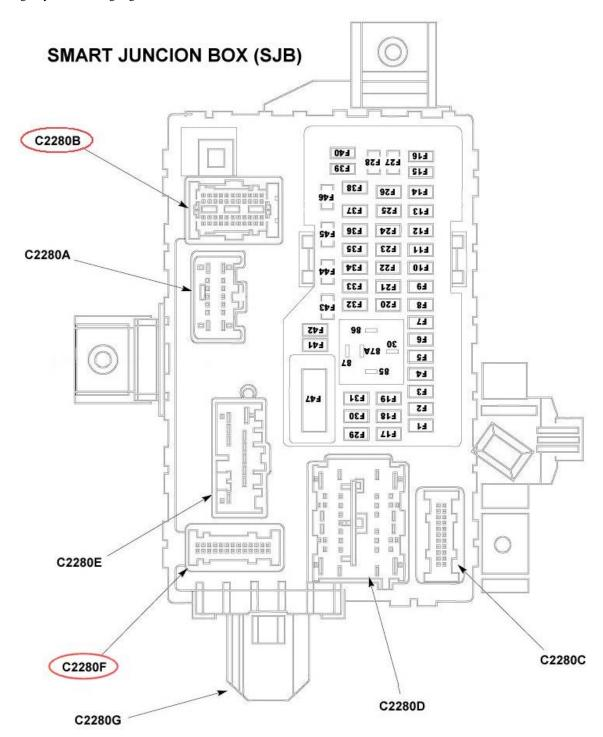
3) Locate and unplug connector C2280F (lower left side in picture above). Unwrap the tape to expose the harness wires.
