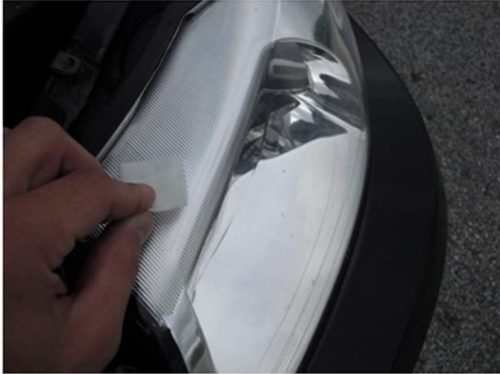
2. Peel backing film from adhesive on light cover.
