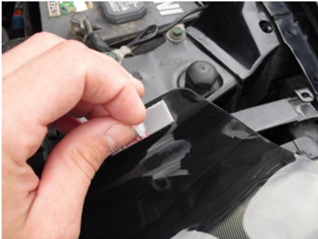
2. Peel backing film from adhesive on light cover.
