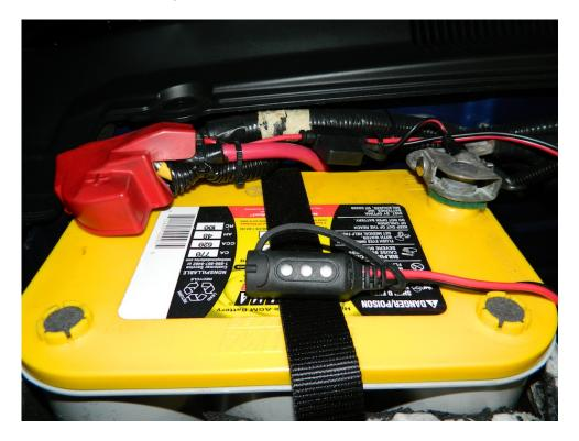
2. Remove rubber protective boot from CTEK connector inlet.
