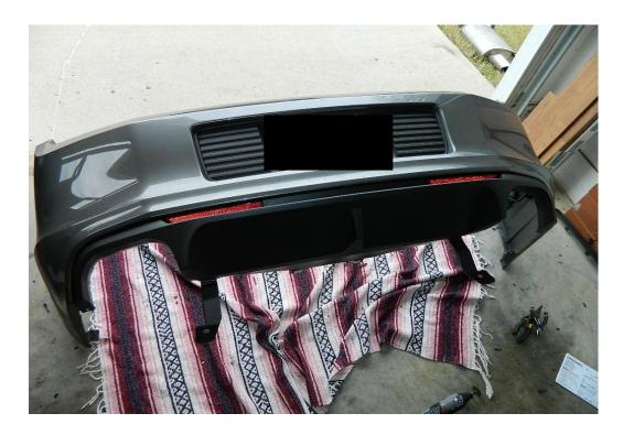
4. With taillights removed (helps a lot) bumper snaps on, from middle to outside. Reinstall rear electrical harness and grommet while snapping bumper back on. <u>Make sure that plastic arms that were uninstalled on old valance are set up to fit between bumper and muffler.</u> If you don't, they will have to be bent to fit, likely resulting in them breaking. (See pic).
