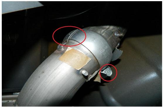
2. Remove rubber holder from muffler. This takes some effort. I used my body to help support the muffler while doing this.
