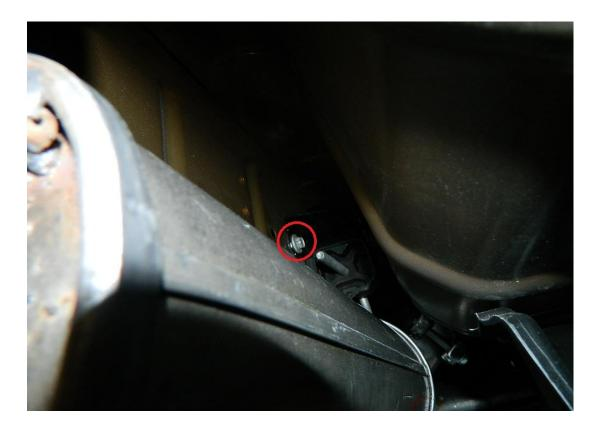
6. Remove mounting bracket from each muffler and transfer to the new mufflers.
