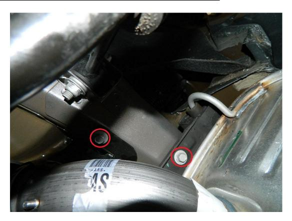
5. Driver side third bolt is difficult to get to, I used the wrench with a regular 13mm socket and pushed the muffler away from the frame to get my hands in. Picture taken from rear of car looking down muffler.
