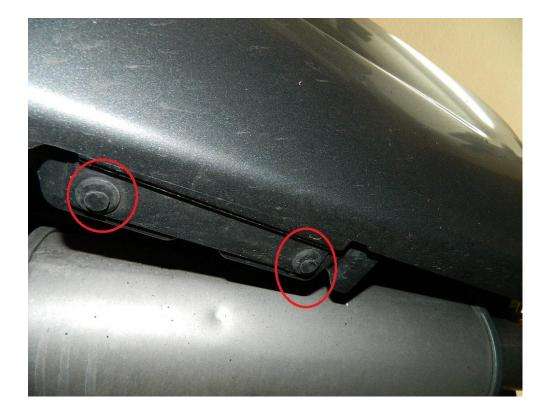
4. Although not necessary, it made it much easier to remove the rear tail lights as well, as the rubber seals along the bumper go up under the lights. (I did not do this until reinstalling the bumper, I should have done it from the start). Remove (1) bolt (13mm) on each side along the cloth of the trunk to get access to all (3) nut/washer sets (11mm) per light. Deepwell sockets are used for the taillights.
