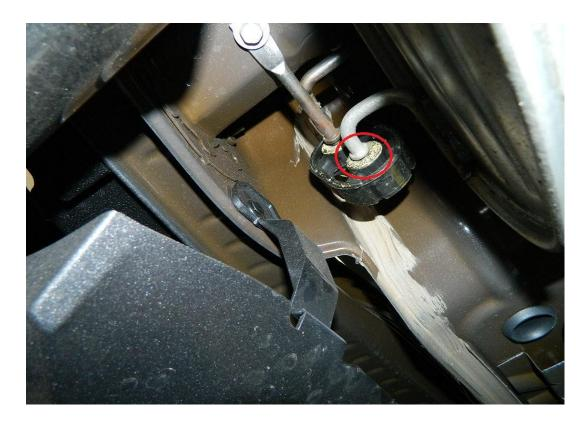
3. Once free, push up on mid pipe and separate ball joint of muffler from pipe. This also takes some effort. (Picture shows bolt still tightened, yours will be loose at this point.)
