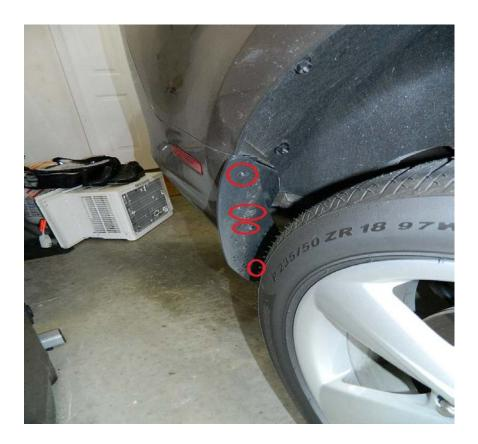
3. Remove (2) pins from under side of bumper that run alongside the mufflers.
