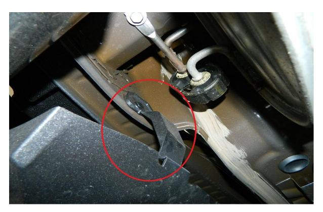
5. Once bumper is snapped on, reinstall push pins on plastic arms and included white plastic locks. Reinstall push pins under side of bumper next to mufflers, and then the rear splash guard and its screws. Reinstall taillights, and then the inner trunk plastic panel.
