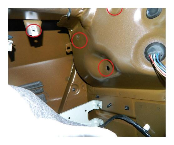
5. Underneath the car, remove (2) push pins and (2) white plastic locks. You will reuse the (2) push pins, but not the white locks. I found the white locks difficult to remove, but since that part of the bumper is getting cut off later, I just broke them to get them out. The new valance comes with its own white plastic locks, so this worked for me.
