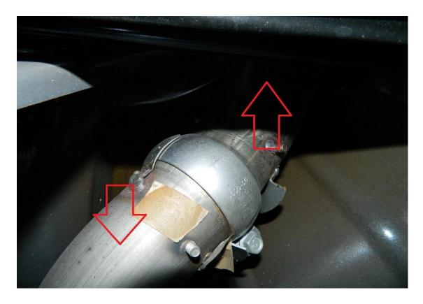
4. Then slide muffler further back along its last set of mounts to make space for removing bolts that secure front muffler bracket. On passenger side there are (2) 13mm bolts, there are (3) on the driver side. Once these are removed, the muffler will fall. Take care to support muffler the whole time.
