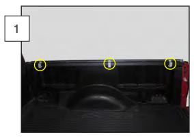
Lay the right side rail onto the right side bed rail. Place 3 clamps along the inside of the rail, making sure not to cover the crossbow cut outs. Repeat on the left side. Loosely snug the brackets.
