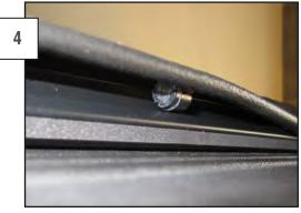
Starting at the front; fold the sides of the tonneau cover down and snap the hidden clips into the side rails, snap them in and work toward the back of the truck, until the entire length is secured. Then secure the snaps along the rear rail. Check for fitment and make sure everything is tight.
