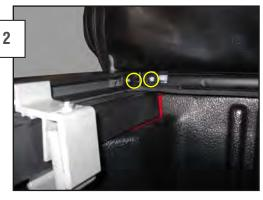
Place the front rail onto the front of the truck. Secure the front rail to both side rails with the corner connector. Insert the phillips screw side into the front bar and the finger knob into each side rail. Tighten down both pieces of hardware. Repeat the same process at the tailgate with the rear rail. Tighten down the 6 side clamps
