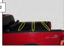
Install the (3) crossbows into the slots on the side rails. With the arc facing upward. Start by inserting the far end into the slot on the side rail then moving the crossbow to the left or right to drop it into the near side rail. Move the crossbow into position. Repeat for all 3. Connect the front of the tonneau cover to the front rail by pressing the hidden buttons into the front rail.
