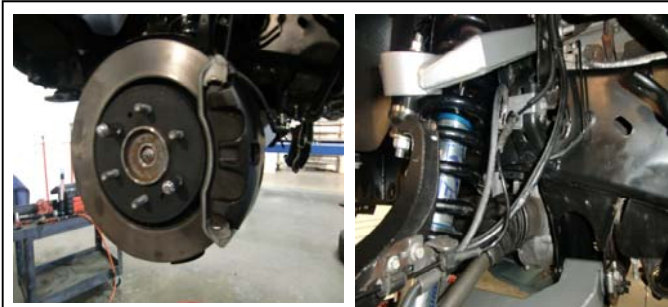
23. Re-install the rotor and brake calipers. Re-attach the ABS lines, brake lines and vacuum line to the spindle.
