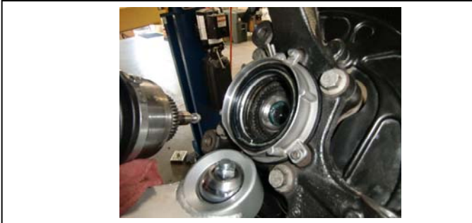
21. Tighten down the top c-lock nut on the LCA uniball. Then re-install the CV joint seal.
