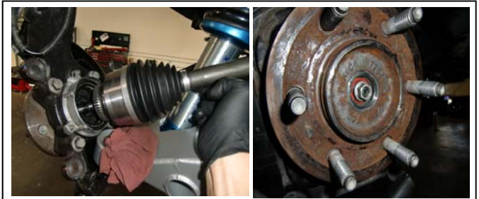
22. Re-install the axle into the spindle. Make sure to line up the teeth. Rotate to ensure that there isn't anything bound up inside. Re-install the nut and the dust seal on the end of the axle.
