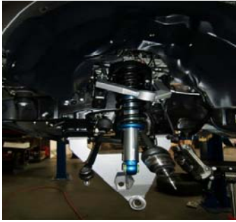
15. Re-install the shock at the top.
