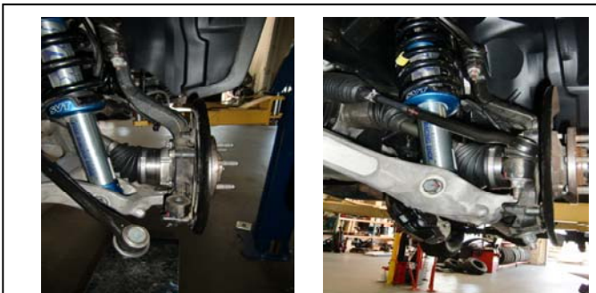
27. Re-attach the tie-rod to the spindle.
