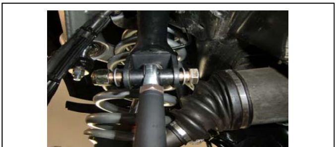
26. Install the sway bar end links to the sway bar bracket. Install the nut to the outside of vehicle
