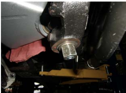
19. Install the spindle onto the LCA. With a washer and a standard nut, tighten the nut down to seat the pin into the spindle.
