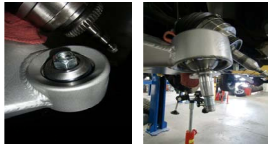
18. Install the misalignment spacers into the LCA uniball. Install the pin with a washer and c-lock nut hand tightened
