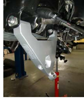
14. Install the ReadyLIFT® lower control arm.
