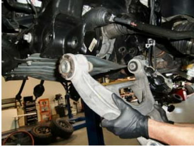
13. Unbolt and remove the lower control arm.
