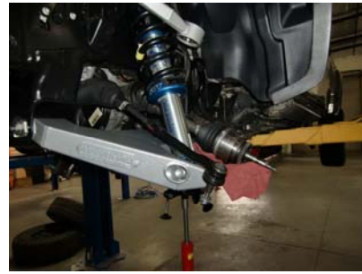
16. Install the lower shock into the lower control arm.
