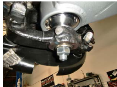
20. Remove the standard nut and replace with a c-lock nut and tighten.
