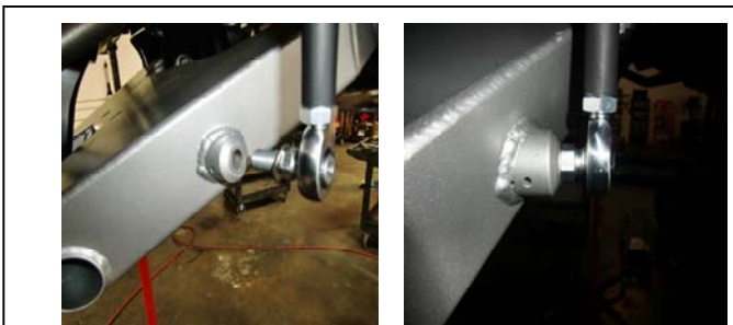
25. Install the sway bar end links to the LCA. Then install the top of the link to the sway bar. If not using Kit # 67-2999 install supplied socket head allen bolt to cap sway bar mount for future use and to protect the thread bung.
