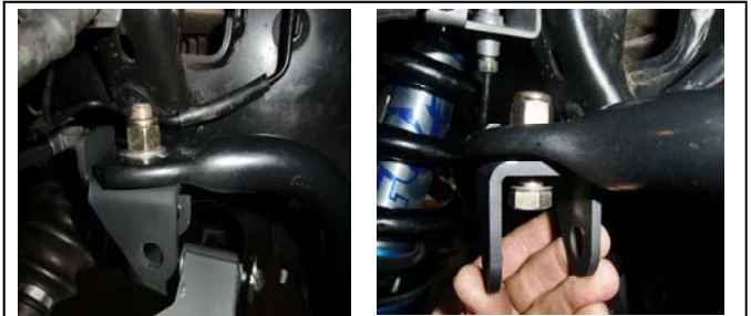
24. To use the factory Sway Bar you must purchase Kit # 67-2999. Install new sway bar end link brackets to the sway bar. If not using factory sway bar this would be the time to remove it from vehicle.
