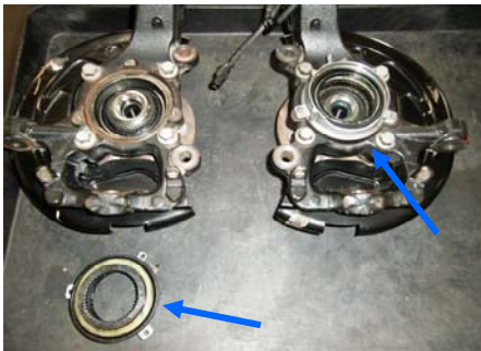
17. Remove the CV joint seal from both of the spindles.
