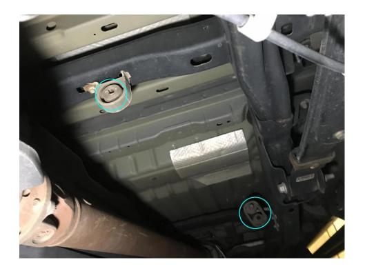
**7.** Bolt new collector to factory Y-pipe (2x13mm Bolts)
