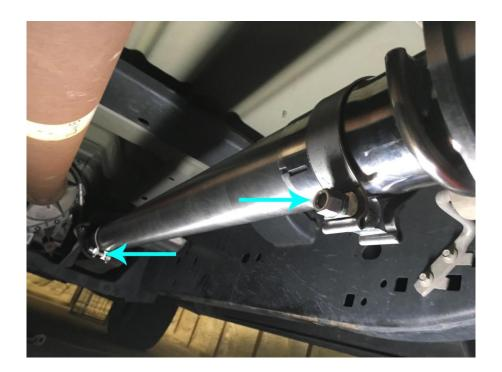
11. Place new rear hanger for tips on suspension bolt (loosen 18mm)
