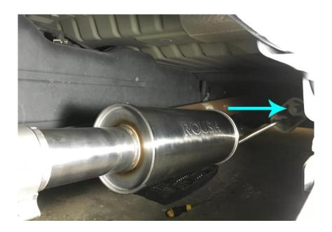
**9.** Place rear pipe over rear end in hangers, and clamp with 3in clamp on front (muffler Side), tighten to snug. (15mm)
