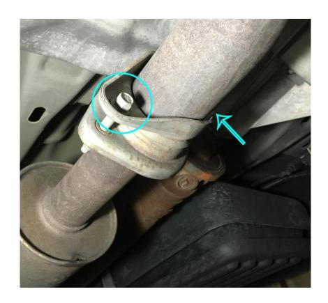
2. Remove Bolt clamping pipe over rear end to Muffler (15mm Bolt)
