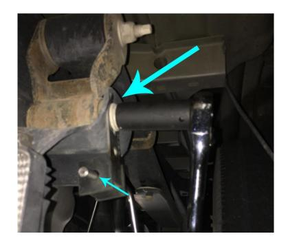
**12.** Clamp Y-Pipe on rear section (2.5 Clamp) and tighten 15mm Bolt Then install the 2 Exhaust Tips and tighten the two 15mm clamps.
