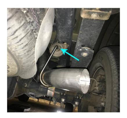
**10.** Test fit mid pipe for size, mark at rear end of pipe, where muffler connects and cut it to size. (Kit fits All Box Sizes) Put clamps both ends of pipe on before putting pipe on, and snug 15mm bolts.
