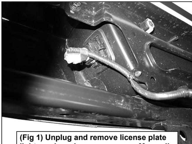
**(Fig 1) Unplug and remove license plate lights and any bumper sensors. Move all wire harnesses away from bumper**
