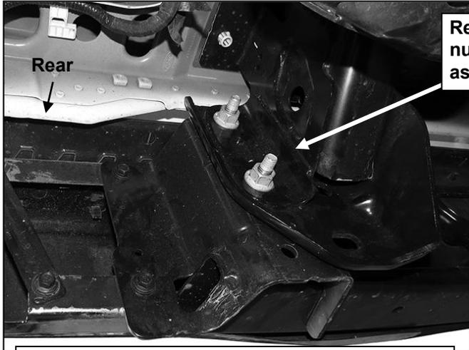
Remove the factory hex nuts attaching bumper assembly to frame
