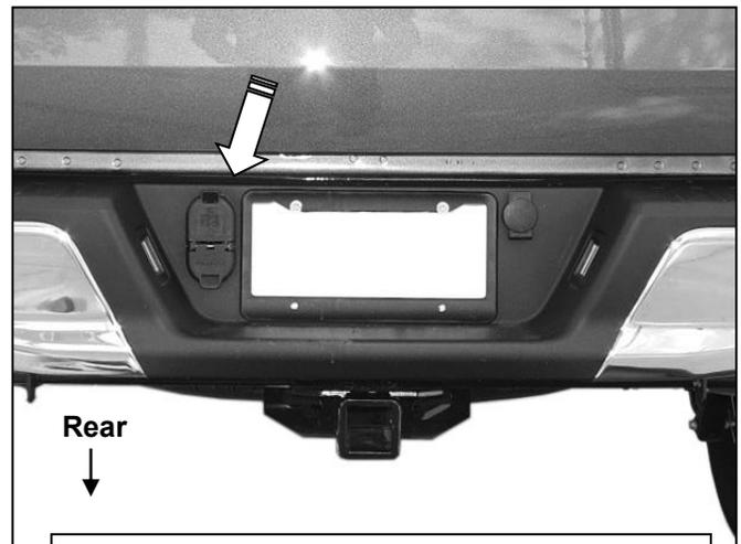
**(Fig 2) Unplug and remove 7-wire trailer plug**
