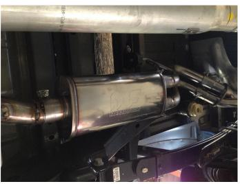
**Step 3.** Install the Muffler Assembly to the Inlet Pipe Assembly using the supplied 3.00" clamp.
